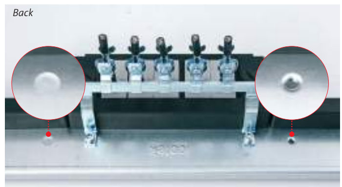
Back Prepared for the assembly of KDR-EMV-PFM. The plates are fitted with threaded screw holes (M5), blocked with plugs. These can be easily removed if necessary. By using the KDR-EMV-PFM, there is no need to additionally install a DIN rail/bus bar above the cable entry, which would otherwise have to be attached in order to implement the EMC connection.
